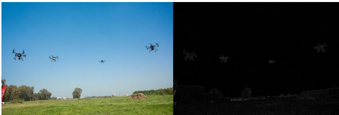
In figure 8 from left to right, the image source is pixabay, the successive images show the Quadcopter, as well as the background edge features, are identified and detected.
