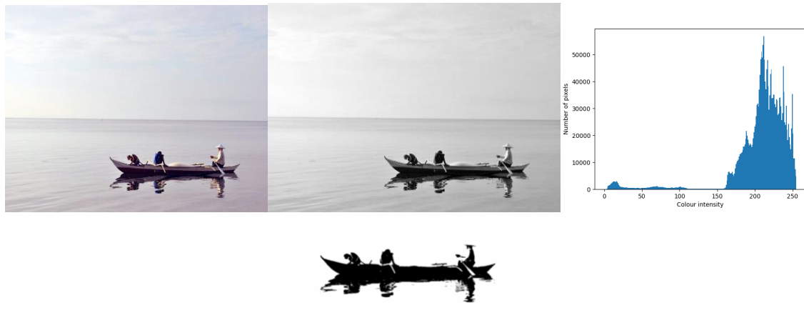
Figure 1 from left to right, the original image; pre-processed image; histogram of the input image; image after thresholding
